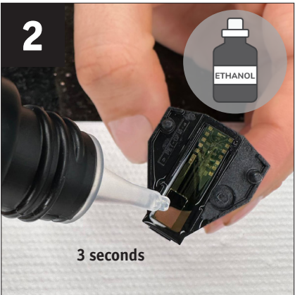
Wet the nozzles with ethanol or moisten a cloth with ethanol. Important: Do not leave it on for more than 3 seconds.
