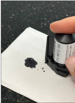
Check if the operation was successful: the cloth should have sucked up the ink from the nozzles, indicated by a black spot on the cloth.
