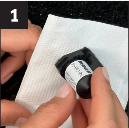
Gently wipe the ink from the nozzles with a lint-free cloth.
